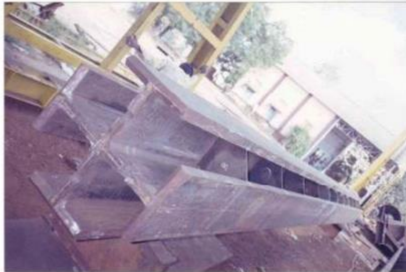
'4' - COLUMN ASSY PROJECT: VINDHYACHAL (NTPC) WT: 125 MT
