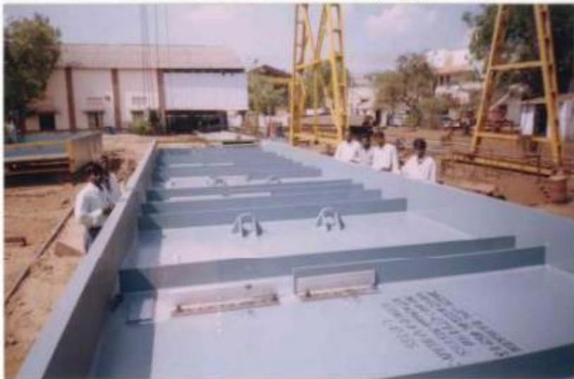
MAIN CEILING GIRDER PROJECT: UNCHHAHAR (NTPC) WT: 49.6 MT
