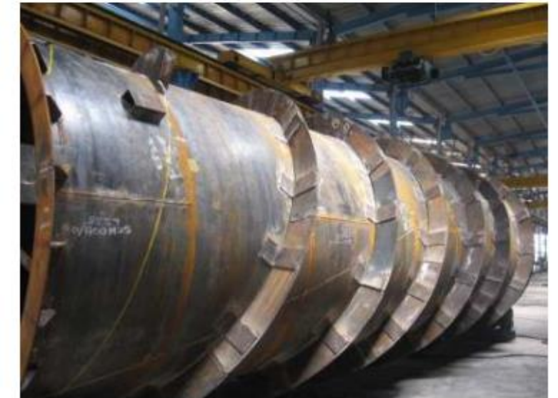
CHIMNEY TRIAL ASSY PROJECT: J.K. TYRE WEIGHT : 65 MT
